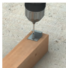
DuraDek stainless steel starter clip fixed using Ø3mm stainless steel screws.
